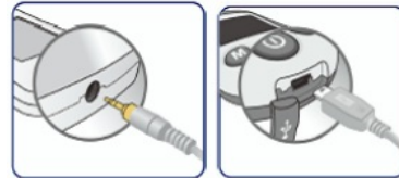
B. Connect to meter's communication port
